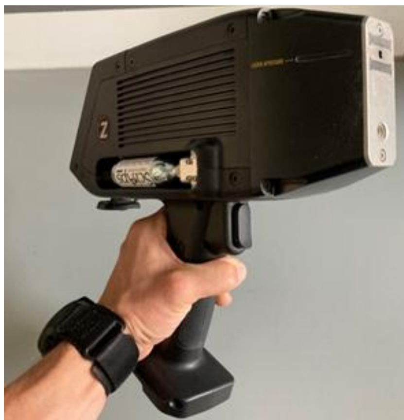
Figure 53: SciAps Z903 handheld LIBS instrument used for the analysis of natural graphite.
