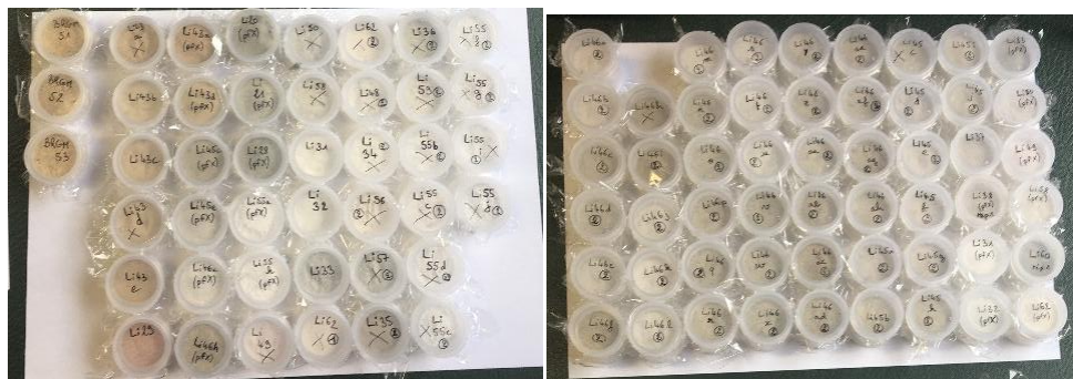
Figure 44: Samples cups with 4 \mu m propylene film used for this study.
