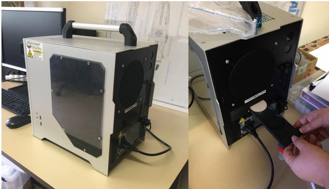
Figure 26: UV bench prototype developed by BRGM/TerraAnalytix. Samples are introduced inside the UV bench using a plastic drawer (right picture).
