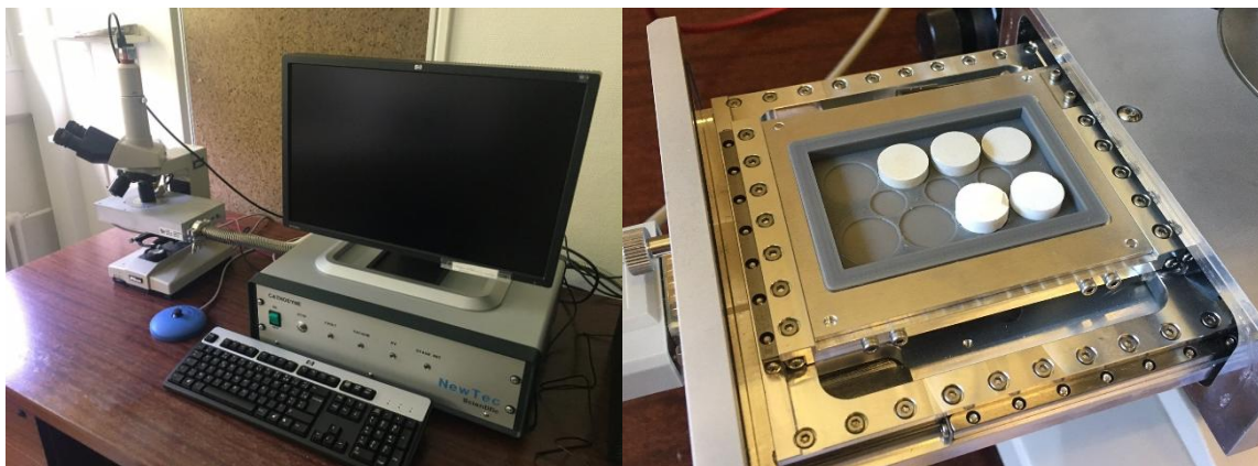
Figure 28: On the left, the Cathodyne cold cathodoluminescence system from NewTec in BRGM laboratories. The system is installed on an optical microscope and linked to a computer and a vacuum pump not visible on the picture. On the right, the custom 3D-printed sample holder in the drawer of the sample chamber.
